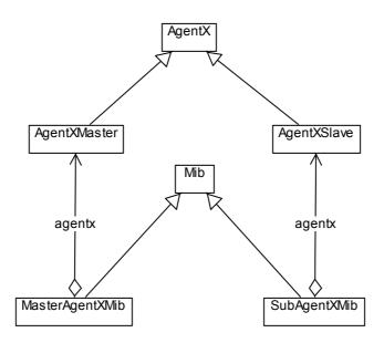
Figure 2: UML Class View of AgentX++ Mib class extensions
