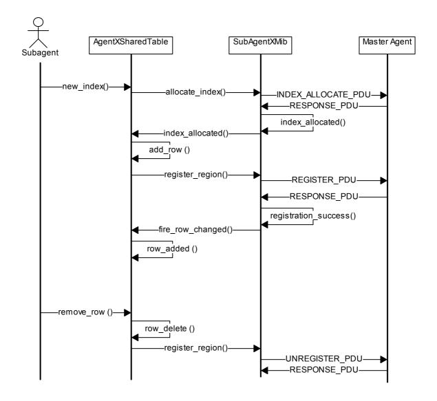
Figure 10: Successful row creation / deletion sequence diagram
