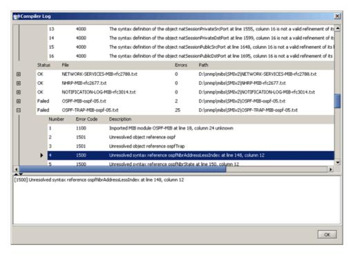
Figure 1: Compiler Log window with compilation errors displayed per MIB module.
