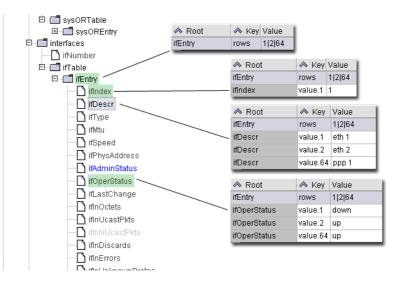
Figure 5: Example properties to simulate table data.
